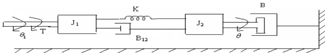
**Q.3** For the mechanical system shown in the figure draw the force-voltage and force-current analogous circuits. 12M
